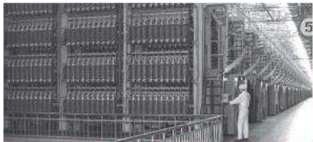
Interior view of a cascade hall of Russia's Novouralsk centrifuge enrichment plant. The facility has a capacity of more than 10 million separative work units per year.
